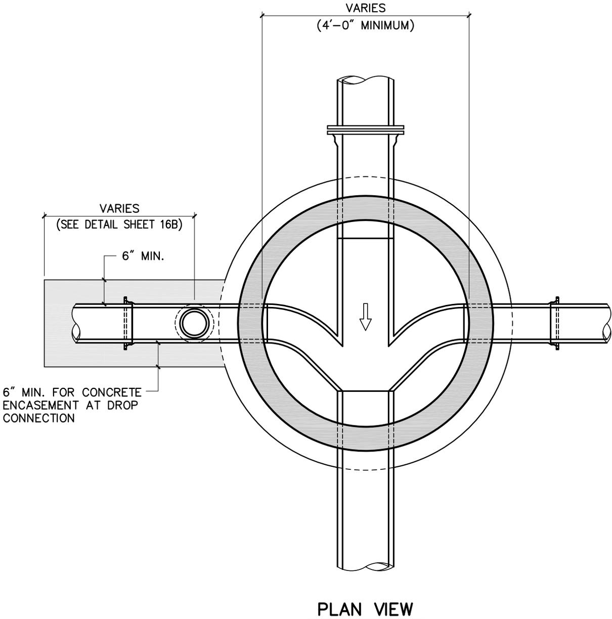
6" MIN. FOR CONCRETE ENCASEMENT AT DROP CONNECTION
