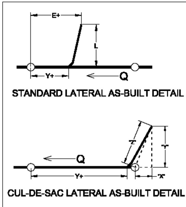
III. Sewer laterals are 6-inch diameter solid wall SDR 26 PVC, unless otherwise noted.
